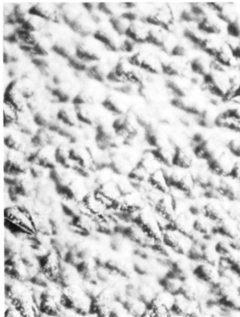
Figure 2. Nomarsky optical microscopic view of polycrystalline \text{CaF}_2 on \text{Si}(100) (magnification \times 400 ).
